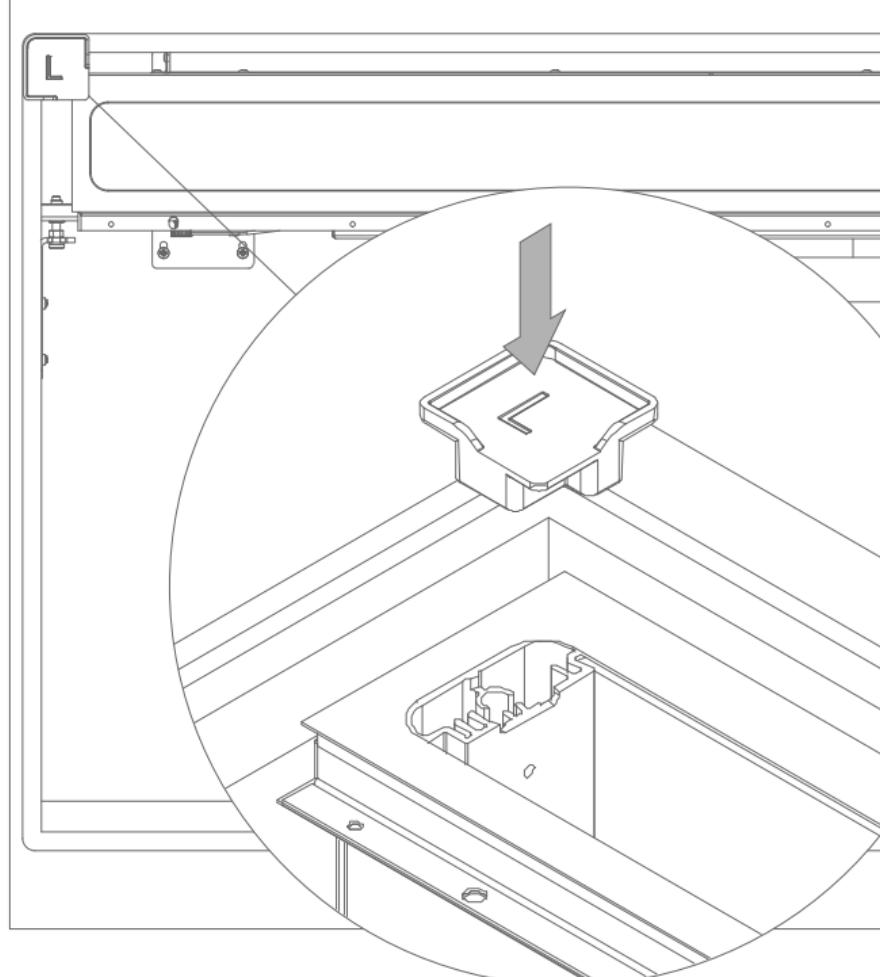
(15) Place the positioning guides (1821135) between the worktop cut-out and the hood.
