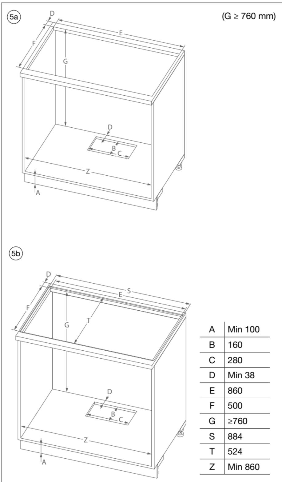
**(5a) Built-in height  $G \geq 760\text{mm}$  surface mounting**
